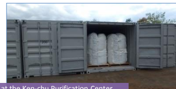
Storage condition of incinerated ash at the Ken-chu Purification Center
