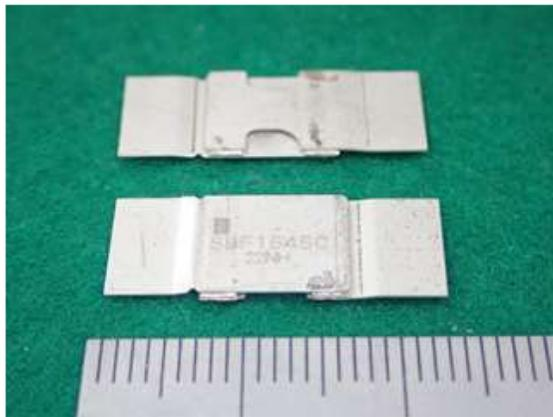
Fig.1 Bypass diode
